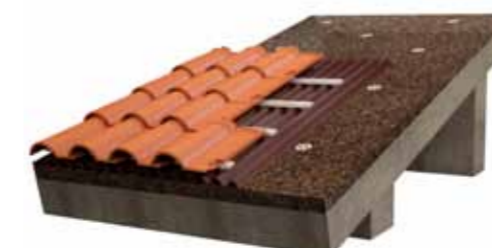
Roofs: Pitched roof with corrugated roofing system
