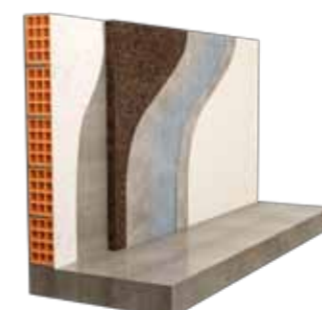
External walls: Interior Insulation
